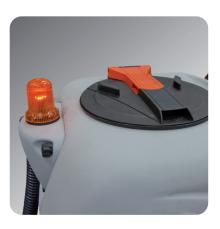
Quick lock recovery tank cap allows for fast and esy cleaning and sanification of the tank; the tilting tank together with a large size drain hose allow the complete emptying of the tank and the removal of any type of solid dirt. The antifoam device protects suction motor, as well as the electronic floating switch that stops suction when the tank is full.
